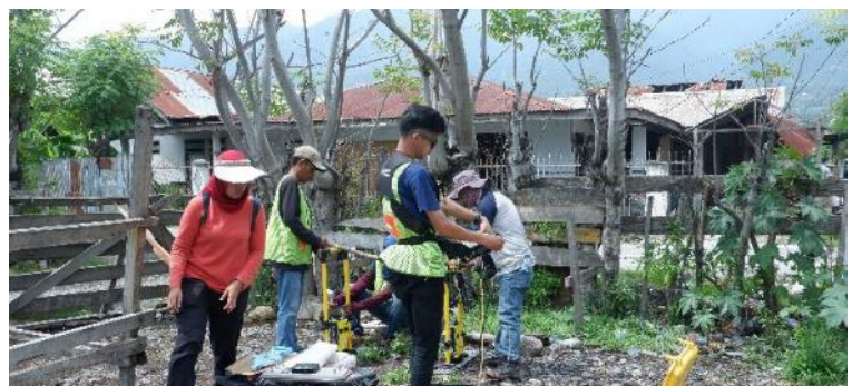
Geological Agency team conducted Multichannel Analysis of Surface Wave (MASW) and Microtremor tests in Palu City, as part of seismic hazard investigation and analysis, which will contribute to a better and safer design of target infrastructures of PETRA. These tests applied in all target locations in Central Sulawesi and West Nusa Tenggara (photo: UNDP)
